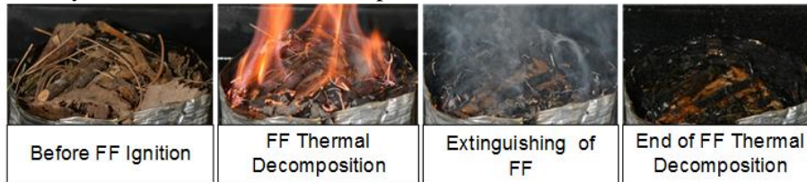
Fig. 2. Video frames of the extinguishing the FF sample (birch leaves; and mixed forest fuels with the following mass ratio: 25% birch leaves; 15% pine needles; 60% branches of hardwoods)
