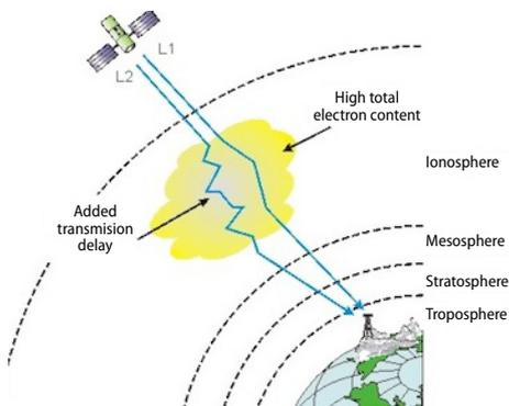
**Figure 1. The L1 and L2 signals broadcast from GPS satellite to reference station**
