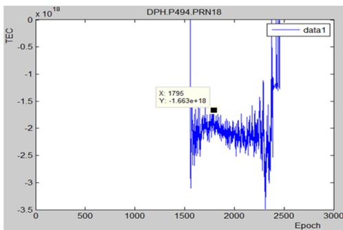
**Figure 10. The TEC deformations are observed in three GPS reference stations for PRN18 satellite in the event day (94); as a significant result is that the epoch number, initial of the deformations, is depend on directly proportional to the distance between earthquake epicenter and station**
