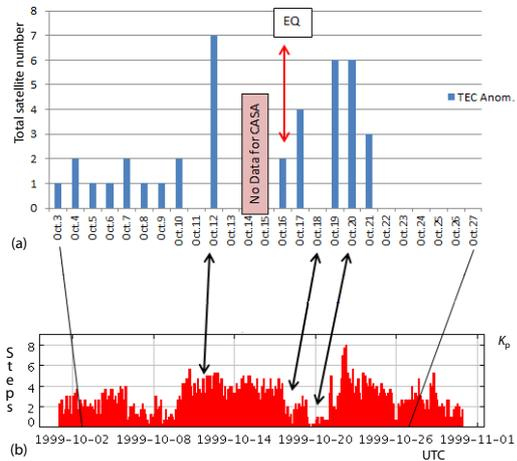
Figure 5. (a) Hector Mine earthquake cumulative TEC anomalies, (b)  $K_p$  index
