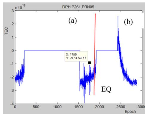
Figure 14. Daily TEC changing chart; there is seen absolute distortion in epoch 1732 before Napa earthquake (1842)
