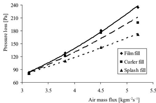
Figure 13. Comparison of pressure loss values for  $G_w = 3.13 \text{ kg/m}^2\text{s}$  and  $L = 0.8 \text{ m}$
