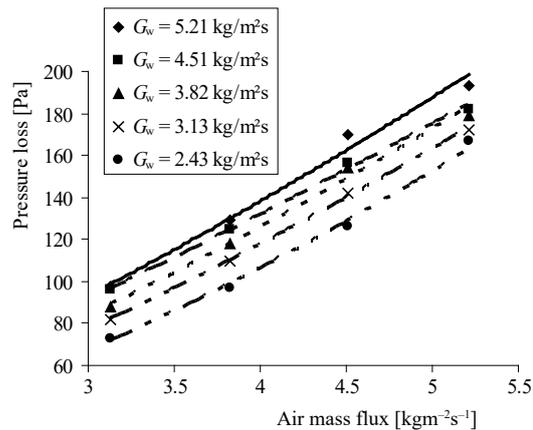
Figure 11. Pressure loss values obtained with splash type fill for 0.8 m fill height
