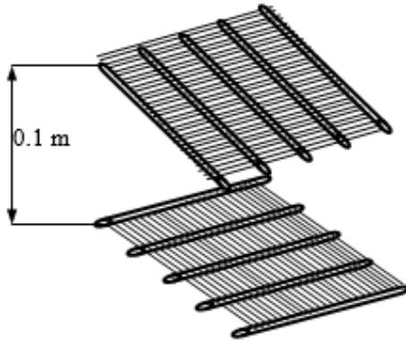
Figure 3. Schematic diagram of splash fill arrangement
