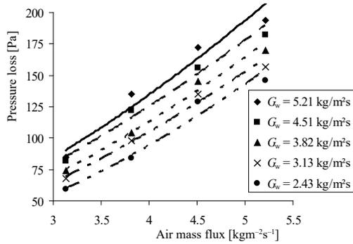
Figure 7. Pressure loss values obtained with curler type fill for 0.6 m fill height
