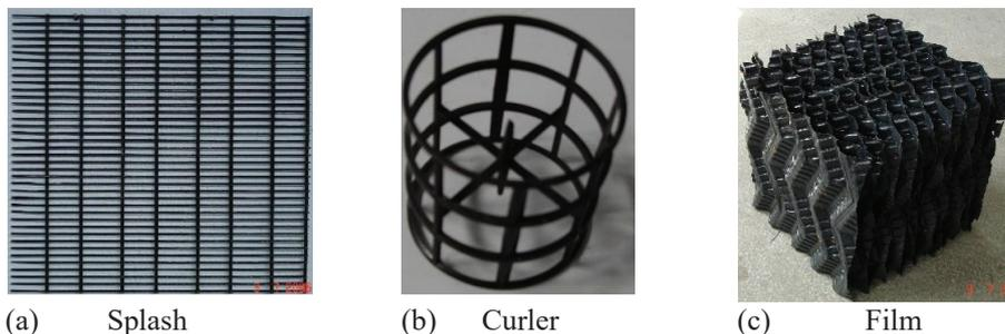
Figure 2. The filling materials used in experimental works
