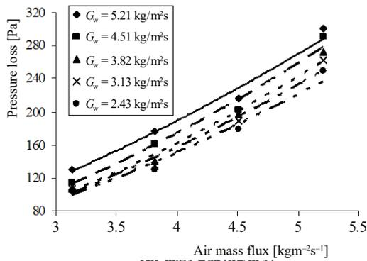
Figure 5. Pressure loss values obtained with film type fill for 0.8 m fill height
