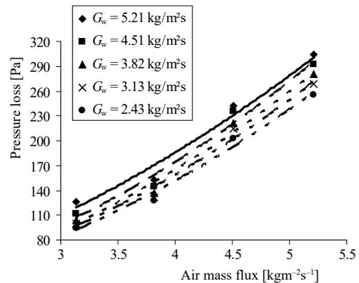
Figure 12. Pressure loss values obtained with splash type fill for 1 m fill height
