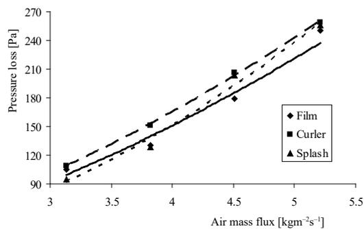
Figure 14. Comparison of pressure loss values for  $G_w = 2.43 \text{ kg/m}^2\text{s}$  and  $L = 1 \text{ m}$
