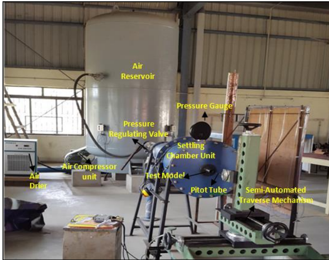
Figure 4. Free Jet Facility at High Speed Jet Laboratory of Rajalakshmi Engineering College
