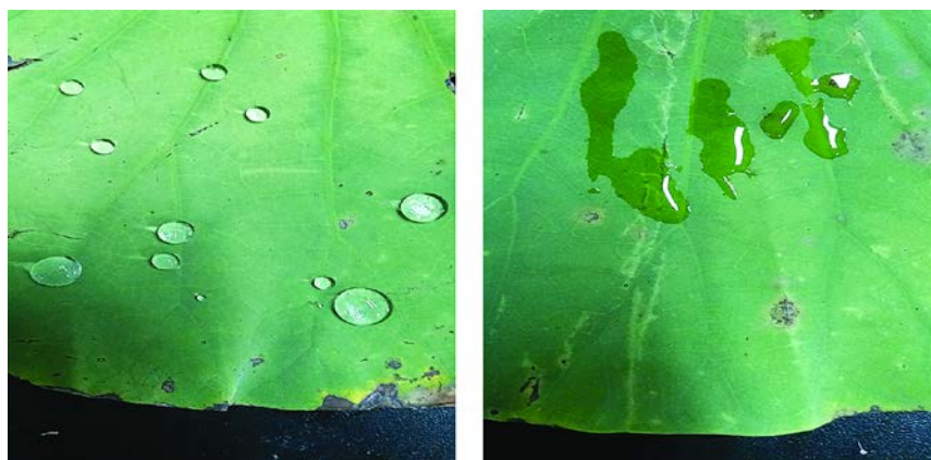
Figure 5. Comparison of water, oil and starch solution on the contact angle on the lotus leaf surface
