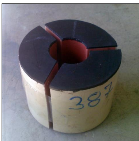
Figure 2. The GMTI base bleed grain used in this study
