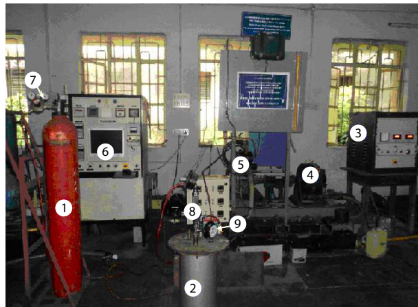
Figure 2. Engine setup; 1 – engine 2 – dynamometer 3 – dynamometer control panel 4 – data acquisition system 5 – hydrogen cylinder 6 – hydrogen pressure regulator 7 – flame trap 8 – hydrogen flow regulator (rotameter) 9 – pressure indicator
