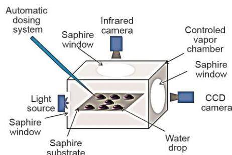
Figure 1. Schema of the experimental set-up
