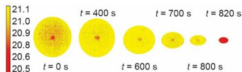
**Figure 5. Snapshots from infrared video camera of evaporation process of water drop until the total disappearance of drop:  $T_{amb} = 21\text{ }^{\circ}\text{C}$  and  $H = 50\%$**
