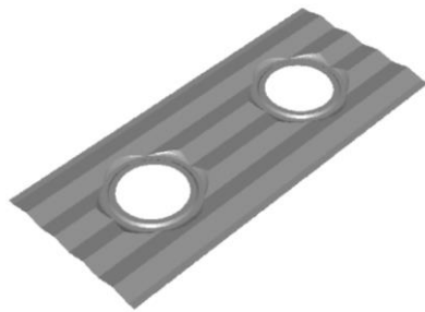
Fig. 1. The schematic diagram of wavy fin (Case 0)
