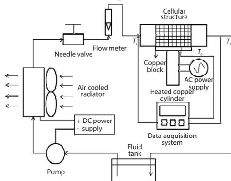
Figure 7. Schematic of experiment set-up
