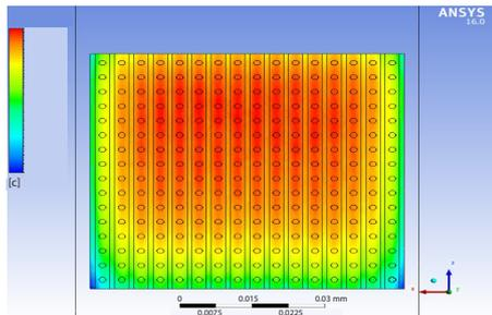
Figure 4. Bottom face temperature distribution at  $0.000025 \text{ m}^3/\text{s}$  (1.5 Lpm)
