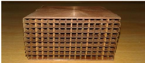
Figure 6. Fabricated micro-hole cellular structure
