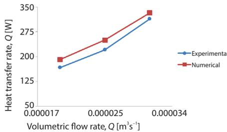
**Figure 10. Variation of heat transfer rate with volumetric flow rate**
