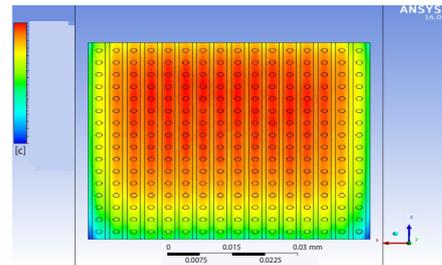
Figure 5. Bottom face temperature distribution at  $0.000034 \text{ m}^3/\text{s}$  (2 Lpm)
