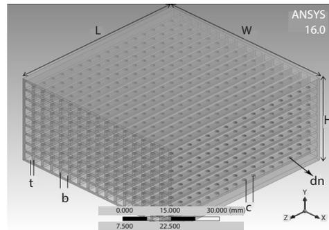
Figure 2. Micro-hole cellular structure
