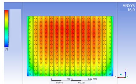
Figure 3. Bottom face temperature distribution at  $0.000017 \text{ m}^3/\text{s}$  (1 Lpm)
