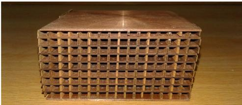
Figure 6. Fabricated micro-hole cellular structure
