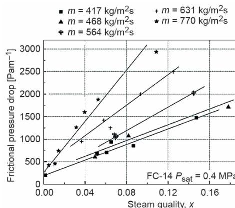
Figure 5. Pressure drop gradient *vs.* flow quality at various mass flux through test Section II
