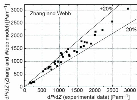
**Figure 7. Comparison between the measured pressure gradient and the predicted results by the Zhang and Webb [6] model**
