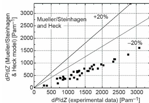
**Figure 8. Comparison between the measured pressure gradient and the predicted results by the Mueller and Heck's [13] model**
