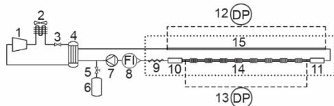
**Figure 1** Schematic diagram of the experimental apparatus and the details of the components; 1 – compressor, 2 – condenser, 3 – throttling valve, 4 – liquefaction heat exchanger, 5 – manual globe valve, 6 – buffer, 7 – magnetic pump, 8 – Coriolis flow-meter, 9 – electric heater (EH), 10-11 – glass tube, 12-13 – 3351 digital pressure (DP) transmitter, 14 – test Section I, 15 – test Section II
