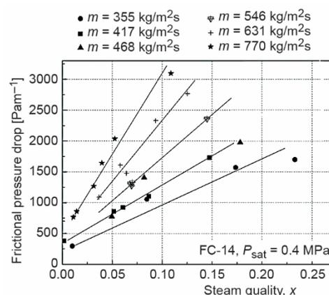
Figure 4. Pressure drop gradient *vs.* flow quality at various mass flux through test Section I
