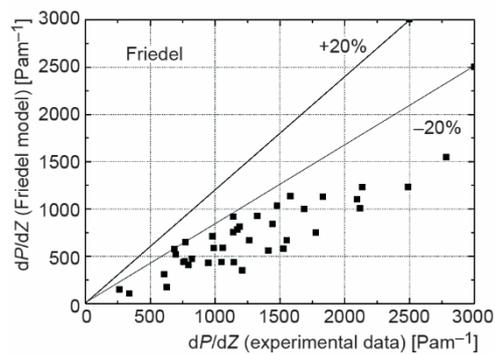
**Figure 6. Comparison between the measured pressure gradient and the predicted results by the Friedel [5] model**
