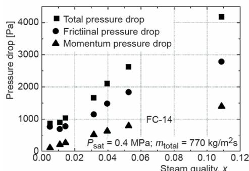
Figure 3. The total pressure drop, frictional pressure drop and momentum pressure drop
