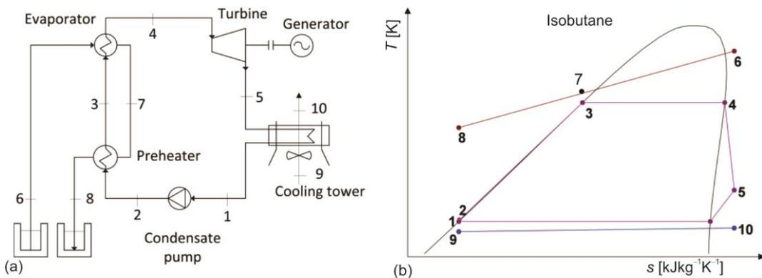
Figure 1. Schematic layout of; (a) simple ORC cycle plant and (b) the associated  $T$ - $s$  diagram
