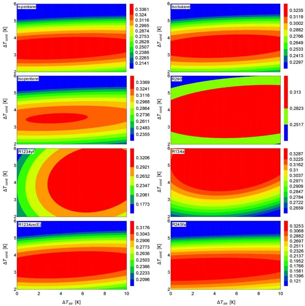
Figure 4. Contours of  $NPI$  as a function of  $\Delta T_{pp}$  and  $\Delta T_{cond}$
