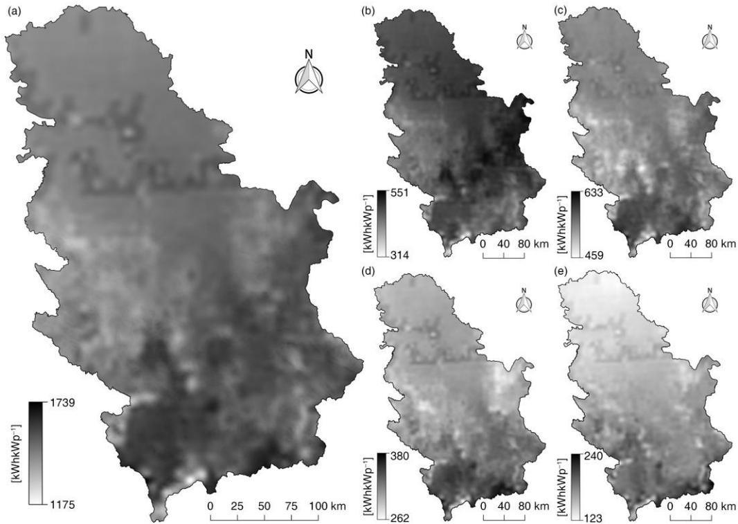
**Figure 2. Electricity generation from a 1 kWp PV system: (a) the average annual values  $[\text{kWhkWp}^{-1}]$ , (b) the average spring values  $[\text{kWhkWp}^{-1}]$ , (c) the average summer values  $[\text{kWhkWp}^{-1}]$ , (d) the average autumn values  $[\text{kWhkWp}^{-1}]$ , (e) the average winter values  $[\text{kWhkWp}^{-1}]$**
