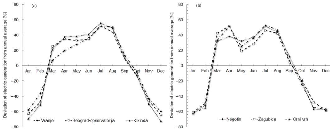
**Figure 3. Monthly deviations of electric generation from annual average [%] for meteorological station: (a) Vranje, Beograd, and Kikinda, (b) Negotin, Žagubica, and Crni vrh**
