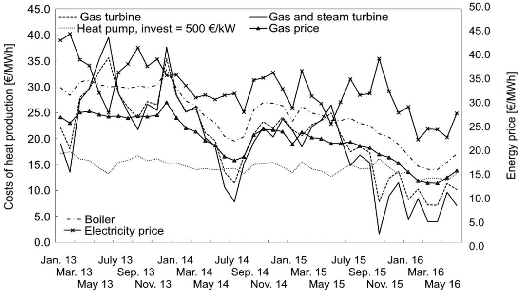
Figure 2. Cumulative costs of heat for a GT, a gas and steam turbine, a boiler and a heat pump system
