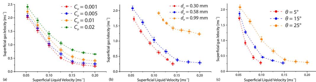
Figure 7. Critical discharge velocity at different experimental conditions; (a) critical discharge velocity at different particle concentrations ( $d_p = 0.58$  mm,  $\theta = 25^\circ$ ), (b) critical discharge velocity at different particle diameters ( $C_p = 0.005$ ,  $\theta = 25^\circ$ ), and (c) critical discharge velocity at different inclination angles ( $d_p = 0.58$  mm,  $C_p = 0.005$ )
