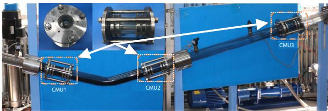
**Figure 3. Conductivity measurement unit**
