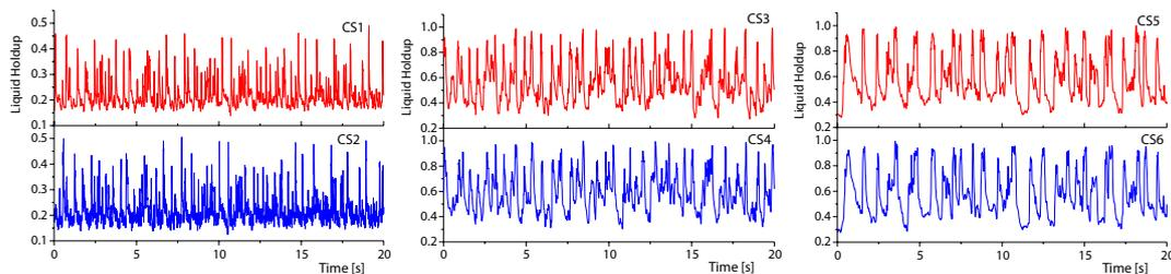
Figure 6. Real-time curves of liquid holdup ( $u_{sg} = 0.87$  m/s,  $u_{sl} = 0.052$  m/s,  $\theta = 25^\circ$ )
