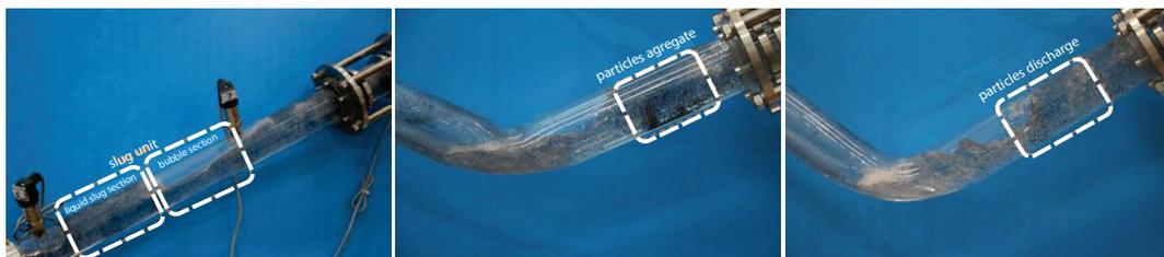
**Figure 5. Flow behavior in the test line**
