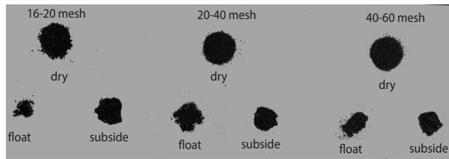
Figure 1. Coal fines samples in different states
