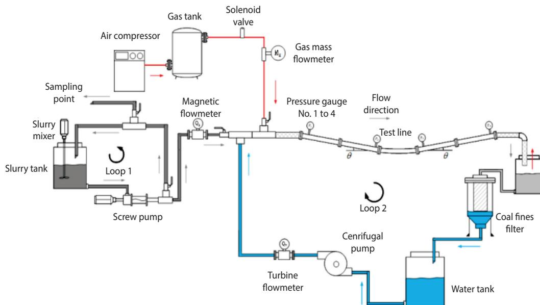
Figure 2. Schematic diagram of gas-liquid-solid three-phase flow experimental apparatus
