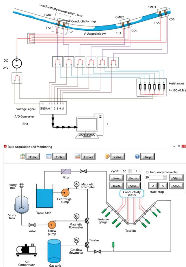
Figure 4. Schematic diagram of conductivity measurement circuit and sync software
