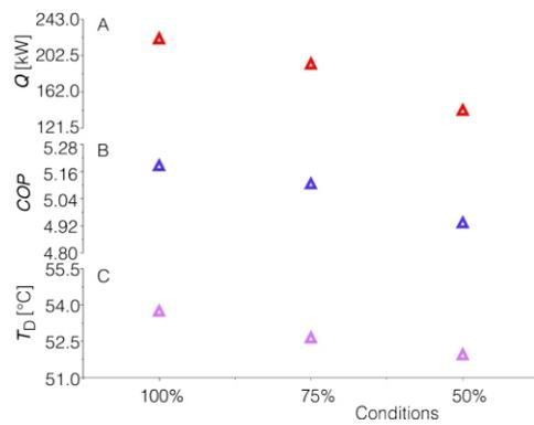
**Figure 4. Performance parameters of original water-cooled screw chiller under different conditions**
