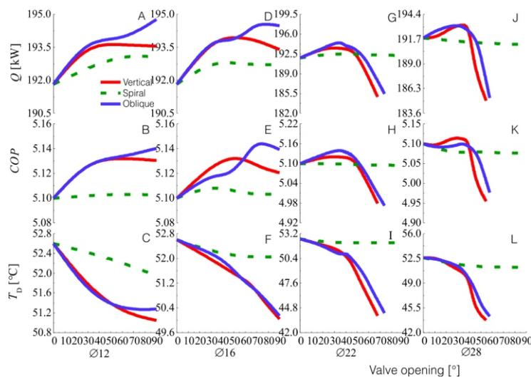
Figure 6. Effect of performance parameters by different diameters and access modes of by-pass tube under load ratio 75% condition
