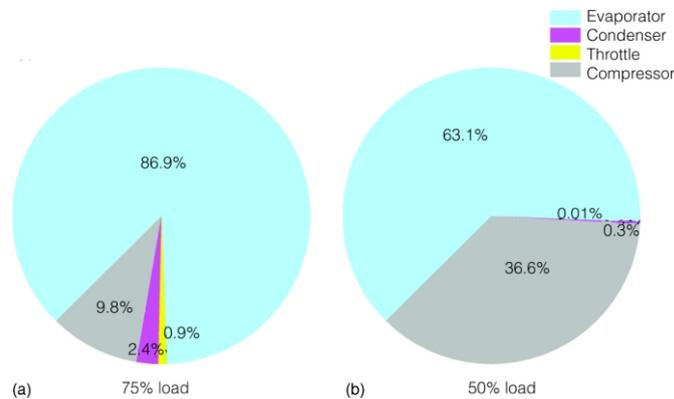
Figure 5. The percentage of exergetic loss of screw chiller main parts under part load state
