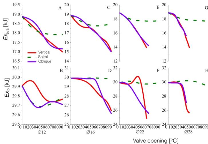
**Figure 9. Effect of exergetic loss of evaporator and ADWC under load ratio 50% condition**
