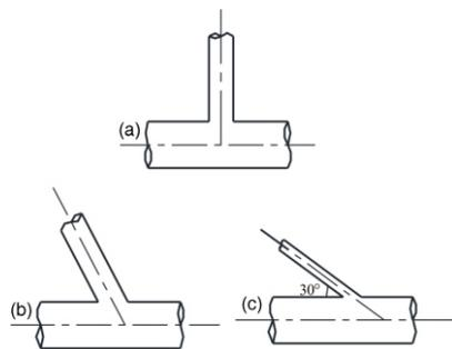
**Figure 2. Access modes of throttle mechanism; (a) vertical access, (b) oblique access, and (c) spiral access**
