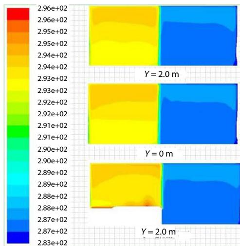
Figure 8. The Y-axis monitoring surface temperature field distribution
