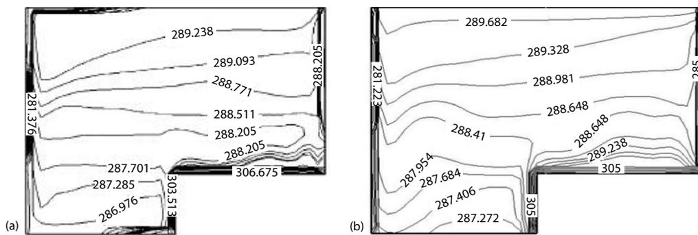
Figure 4. Comparison of temperature field of  $Z = 2$  m cross-section in kang heating room; (a) literature, (b) verification
