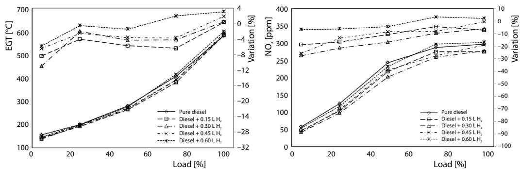
Figure 4. Variation of EGT (a), and NO<sub>x</sub> emissions (b)
