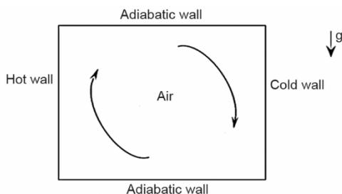
Figure 2. Geometry of a square cavity differentially heated [21]
