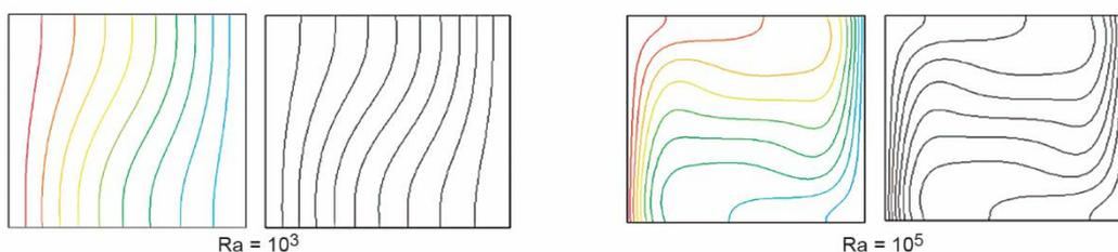
**Figure 3.** Comparison of the isotherms obtained in the present work and those obtained by [20]; (a) present work, (b) results of [20] (for color image see journal web site)
