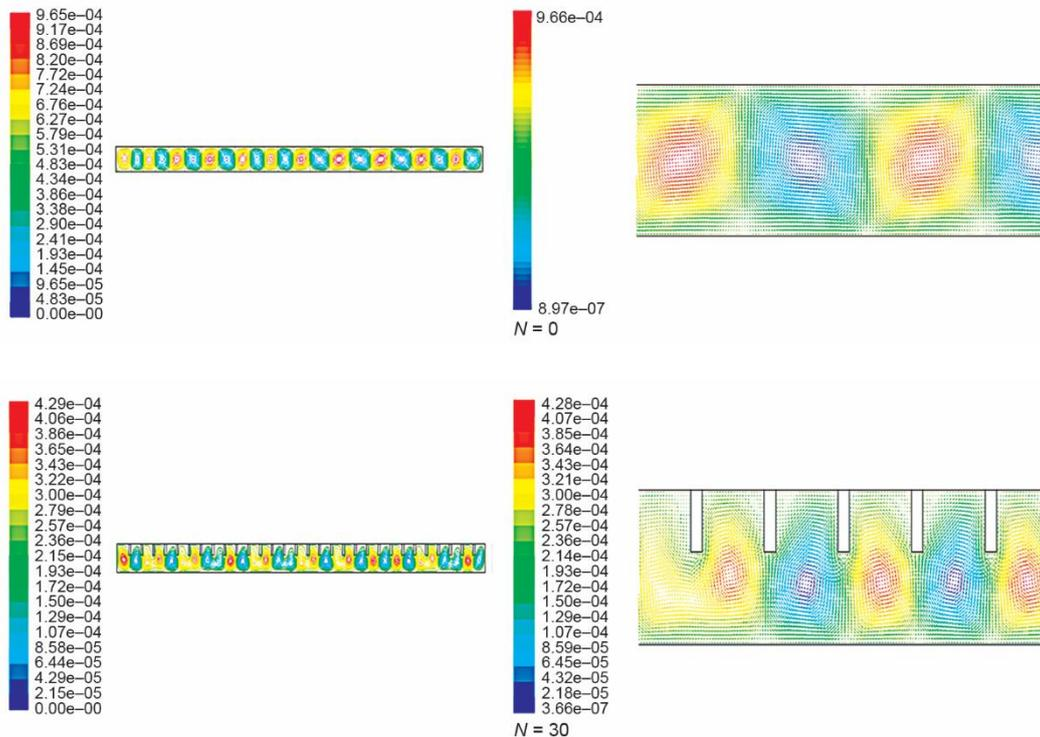
**Figure 9. Streamlines and velocity vectors for different values of the number of partitions  $N$ , for  $Ra = 2.51 \cdot 10^4$ ,  $L_p = 0.4$  (for color image see journal web site)**
