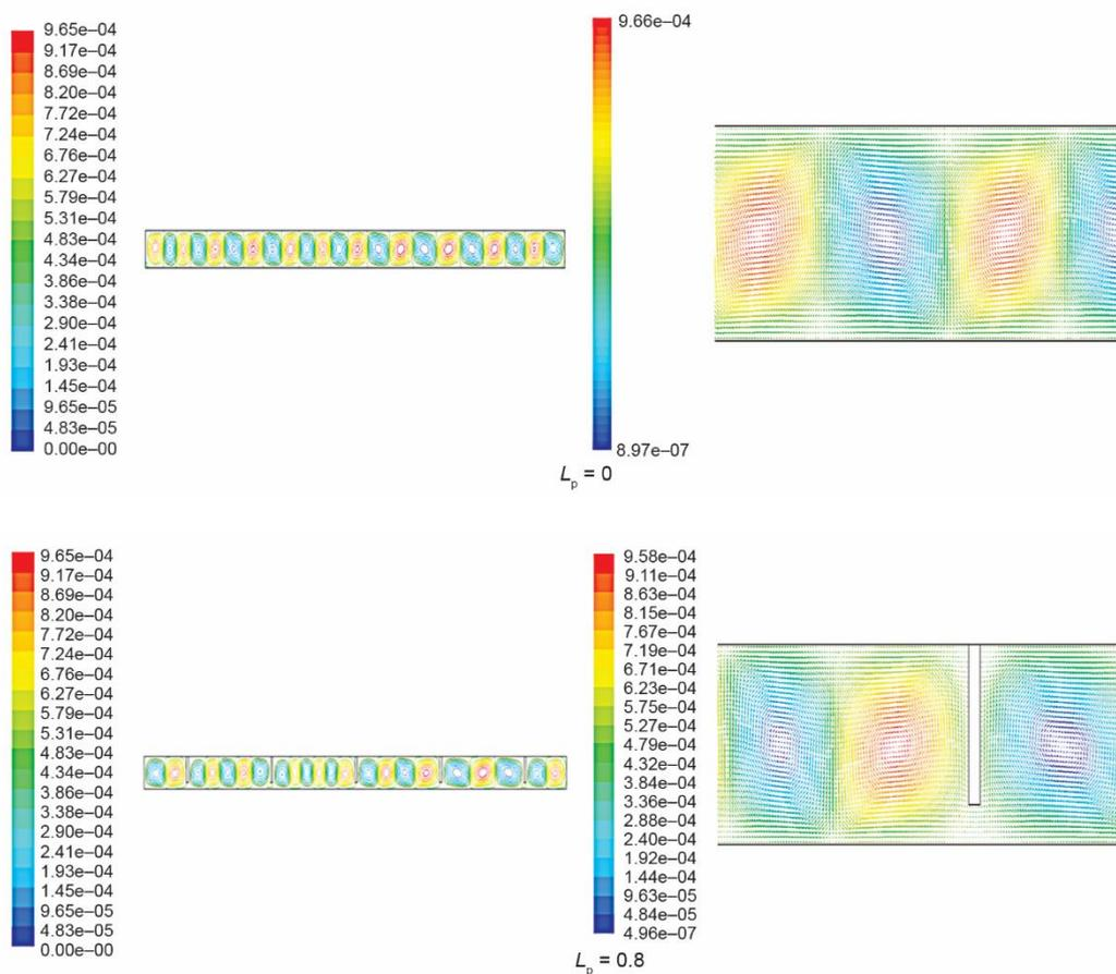
**Figure 6. Streamlines and vectors velocity for different values of  $L_p$ , for  $Ra = 2.51 \cdot 10^4$ ,  $N = 5$  (for color image see journal web site)**
