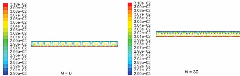
**Figure 8. Isotherms for different values of the number of partitions  $N$  for  $Ra = 2.51 \cdot 10^4$ ,  $L_p = 0.4$  (for color image see journal web site)**
