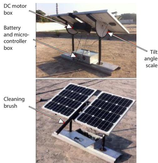
**Figure 6. Experimental set-up of proposed SCM (front and rear side of PV panel pair having SCM)**
