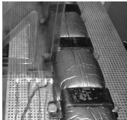
Figure 3. Thermocouples positions on the perforated plate
