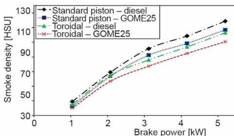
Figure 11. Brake power vs. smoke density
