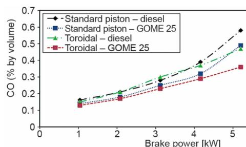
Figure 8. Brake power vs. carbon monoxide
