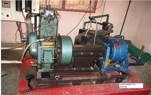
**Figure 3. Photographic view of the Kirloskar TV-1 engine**
