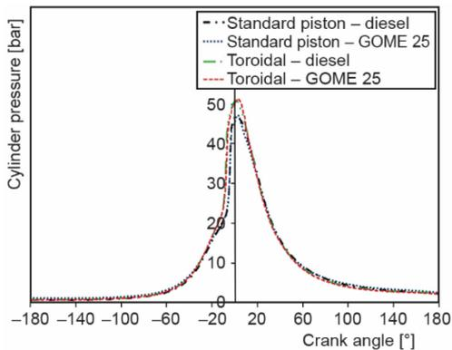
Figure 6. Crank angle vs. cylinder pressure
