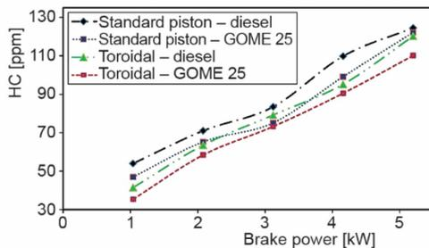
Figure 9. Brake power vs. unburned hydrocarbon
