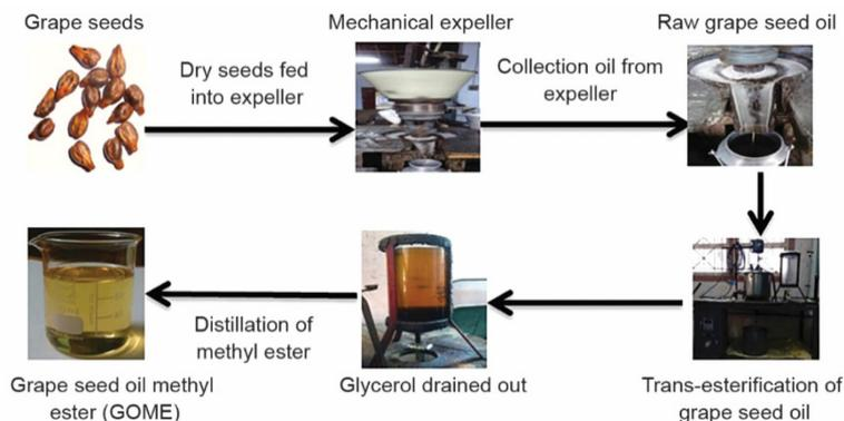
Figure 1. Generation of grape seed oil methyl ester GOME flow chart
