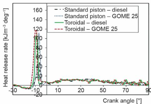
Figure 5. Crank angle vs. heat release rate
