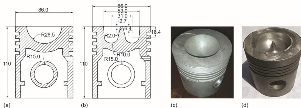
**Figure 4.** Piston details; (a), (b) schematic diagram different combustion chamber geometries, (c), (d) photographical view of different combustion chamber geometries; (a), (c) standard piston combustion chamber; (b), (d) toroidal combustion chamber; dimensions in mm
