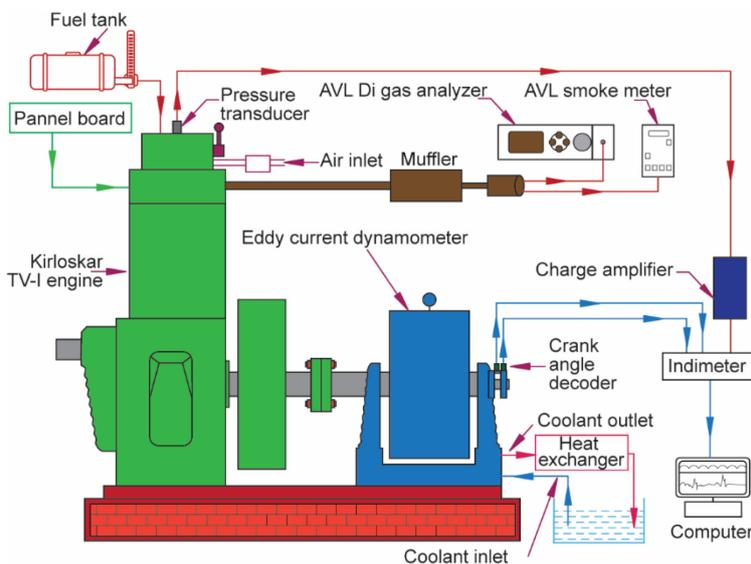
Figure 2. Schematic drawing of the investigational set-up
