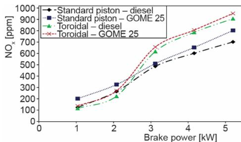
Figure 10. Brake power vs. NO<sub>x</sub>
