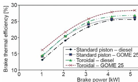
Figure 7. Brake power vs. brake thermal efficiency
