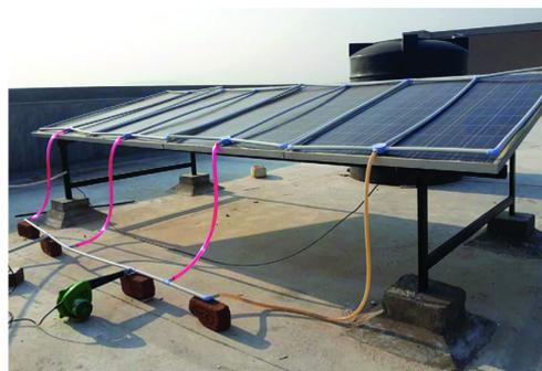
**Figure 2. Photographic view of cooling arrangement**
