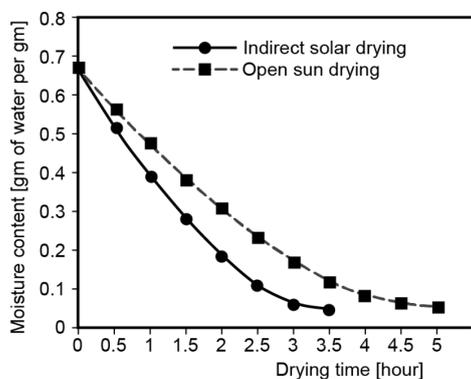
Figure 3. Variation of moisture content (w.b) of curry leaves during drying time
