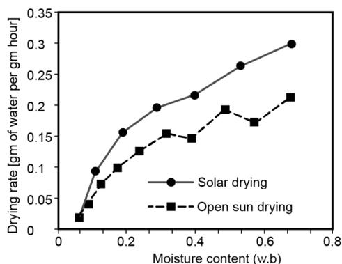
Figure 5. Variation of drying rate of curry leaves with moisture content (w.b)
