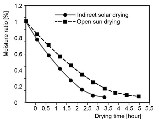
Figure 4. Variation of moisture ratio ( $MR$ ) of curry leaves during drying time
