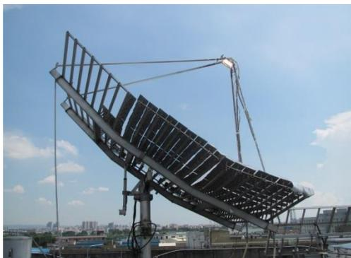
Figure 1. A high concentration PV system with plane mirrors array
