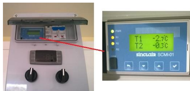
Figure 4. PID control unit of the DC inverter refrigerator
