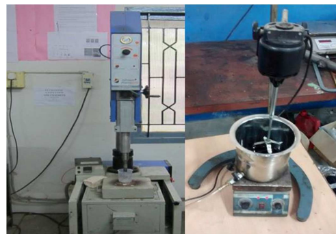
Figure 2. Ultrasonic agitator and mechanical stirrer arrangement
