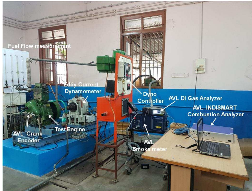
Figure 3. Photographic view of the test engine setup
