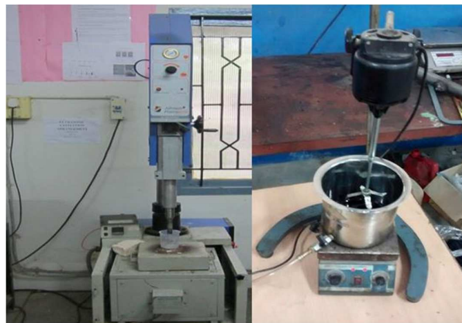
Figure 2. Ultrasonic Agitator and Mechanical Stirrer arrangement
