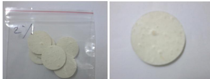
Figure. 2 Preparation of propellant pellet samples using die press
