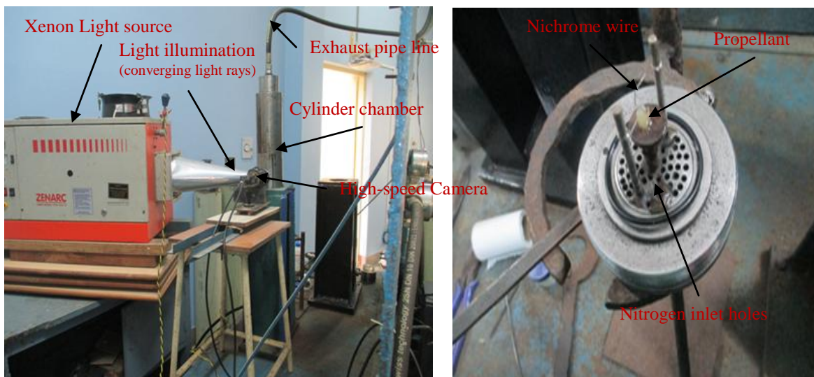
Figure. 3 Experimental view of the window bomb set-up
