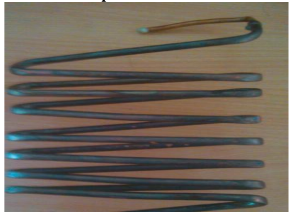
Figure 4. coated heat exchanger coil
