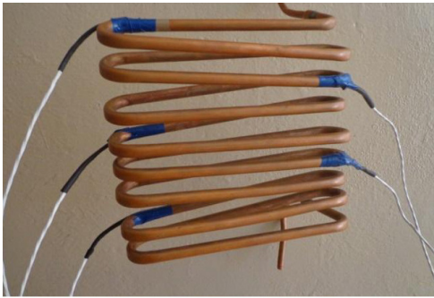
Figure 3. Uncoated heat exchanger coil
