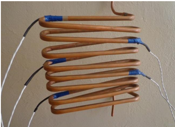
Figure 3. Uncoated heat exchanger coil
