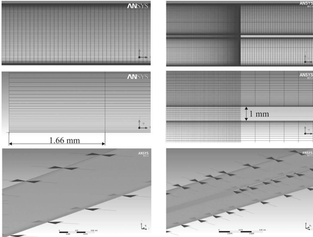
**Figure 2. Mesh of computational domains (left-flow domain, right-flow domain with flat plate)**
