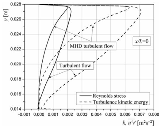
**Figure 11.** Influence of magnetic field on turbulent kinetic energy and Reynolds stresses ( $x/L = 0$ ) (for color image see journal website)
