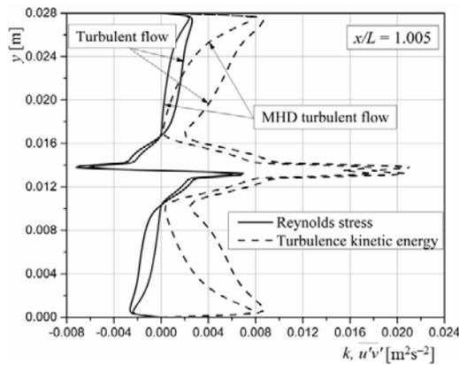
**Figure 17. Turbulence kinetic energy and Reynolds stresses in wake region** (for color image see journal website)
