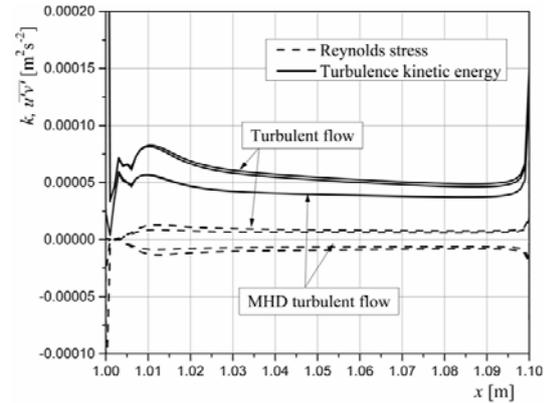
**Figure 18. Turbulence kinetic energy and Reynolds stress along the flat plate** (for color image see journal website)
