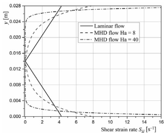
**Figure 5. Influence of Hartmann number on shear strain rate**
