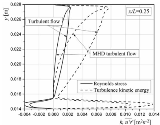
**Figure 12.** Influence of magnetic field on turbulent kinetic energy and Reynolds stresses ( $x/L = 0.25$ ) (for color image see journal website)
