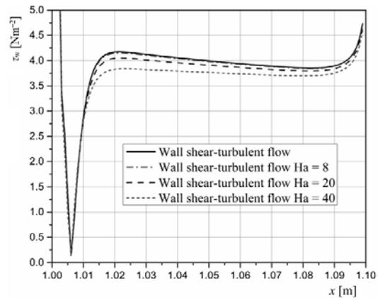
**Figure 20. Wall shear along the flat plate** (for color image see journal website)
