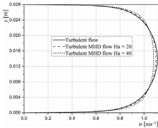
Figure 7. Influence of Hartmann number on longitudinal velocity component
