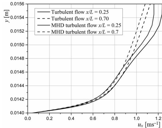
**Figure 16. Boundary layer velocity for turbulent and MHD turbulent flow** (for color image see journal website)
