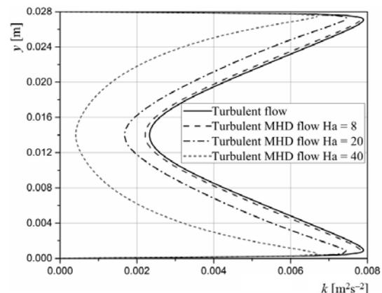
Figure 10. Influence of Hartmann number on turbulent kinetic energy
