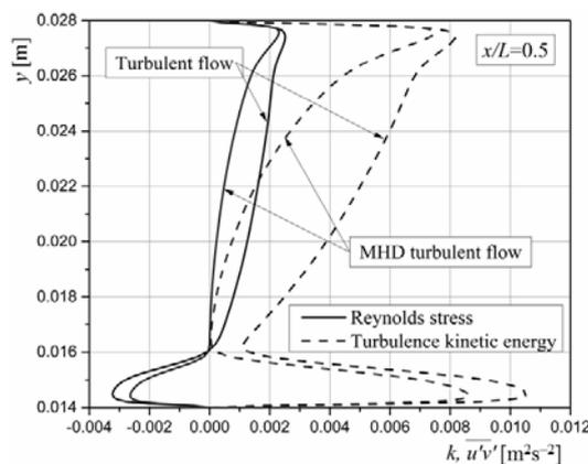
**Figure 13.** Influence of magnetic field on turbulent kinetic energy and Reynolds stresses ( $x/L = 0.5$ ) (for color image see journal website)
