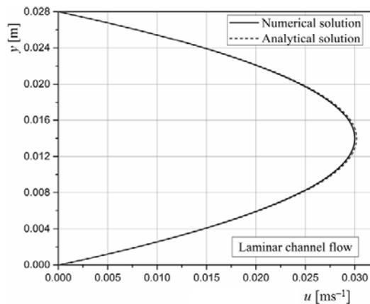
Figure 3. Laminar flow velocity distribution
