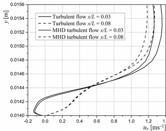
**Figure 15. Boundary layer velocity for turbulent and MHD turbulent flow** (for color image see journal website)
