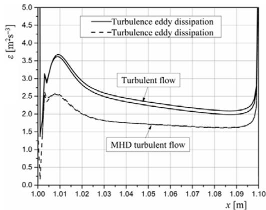
**Figure 19. Turbulence eddy dissipation along the flat plate** (for color image see journal website)
