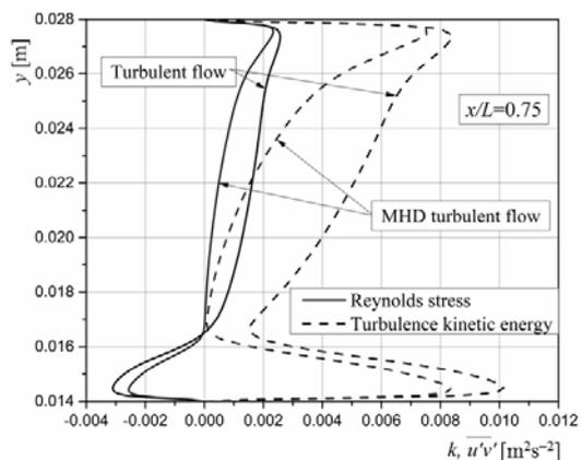
**Figure 14.** Influence of magnetic field on turbulent kinetic energy and Reynolds stresses ( $x/L = 0.75$ ) (for color image see journal website)
