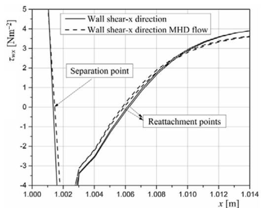
**Figure 22. Wall shear in separation zone** (for color image see journal website)
