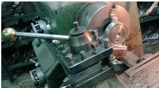
Figure 5. The bearing driven by the lathe electromotor [16]
