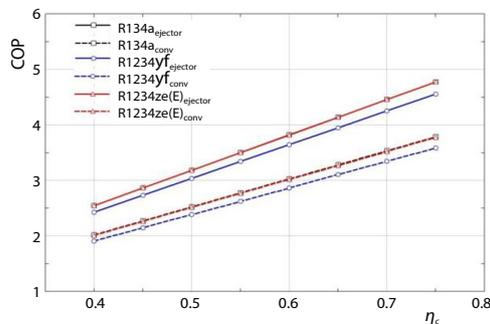
Figure 6. Effect of compressor efficiency on COP
