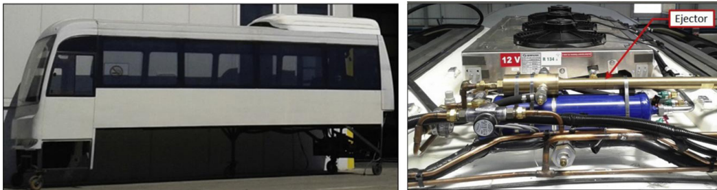
Figure 3. Ejector refrigeration system for bus
