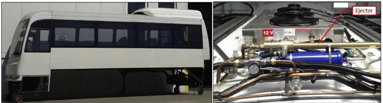
Fig. 3. Ejector refrigeration system for bus
