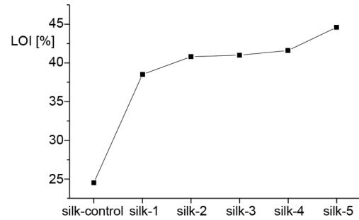
Figure 1. The LOI value curve of the treated and untreated samples
