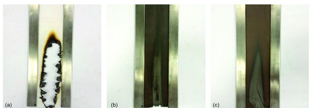
Figure 2. Vertical flame test images of silk-control (a), silk-1 (b), and silk-5 (c)
