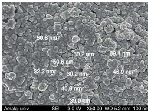
Figure 4. Scanning electron micrograph of synthesized ceria nanoparticles
