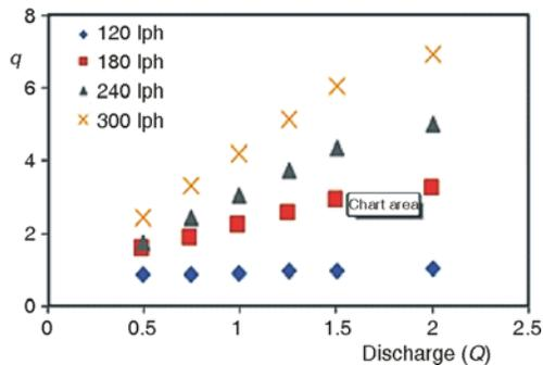
Figure 14. Discharge ( $Q$ ) vs. heat transfer rate ( $q$ )
