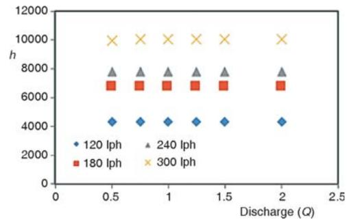
Figure 13. Discharge ( $Q$ ) vs. heat transfer coefficient ( $h$ )
