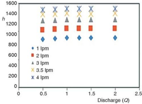
Figure 9. Discharge ( $Q$ ) vs. heat transfer coefficient ( $h$ )
