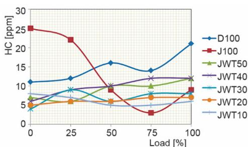
Figure 7. The HC vs. load
