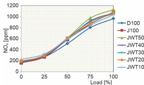
Figure 9. The NO<sub>x</sub> vs. load
