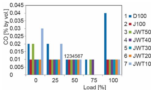
Figure 6. The CO vs. load
