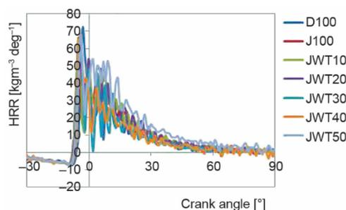
Figure 12. The HRR vs. load
