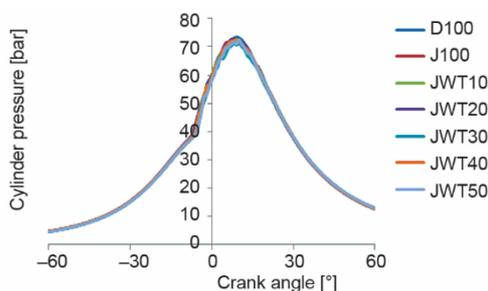
Figure 11. Cylinder pressure vs. crank angle
