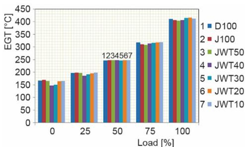
Figure 5. The EGT vs. load
