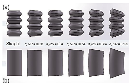
Figure 1. Tested segments of Archimedean spiral coil
