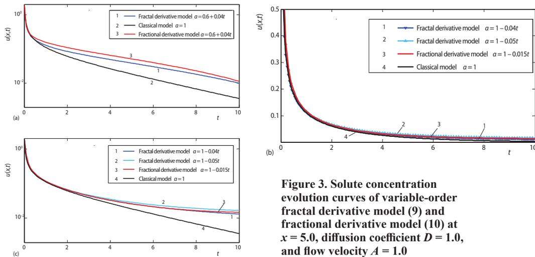
**Figure 3.** Solute concentration evolution curves of variable-order fractal derivative model (9) and fractional derivative model (10) at  $x = 5.0$ , diffusion coefficient  $D = 1.0$ , and flow velocity  $A = 1.0$
