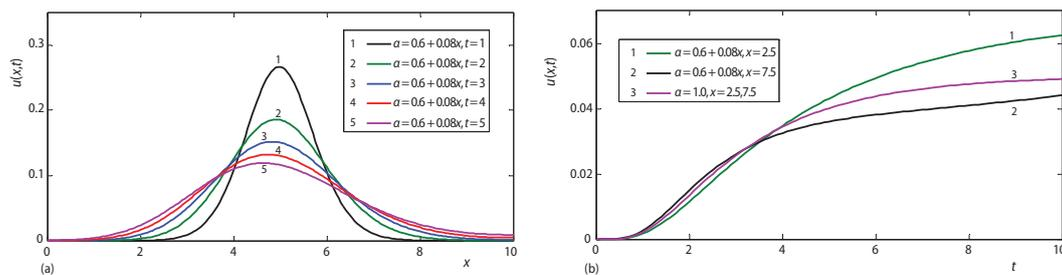
**Figure 2. Solute diffusion curves obtained by using variable-order fractal derivative diffusion equation model (9) with diffusion coefficient  $D = 1.0$**
