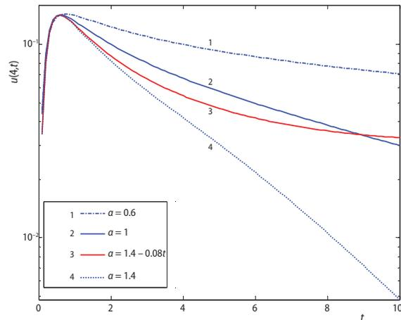
**Figure 1. The dimensionless breakthrough curves of fractal derivative model at spatial location  $x = 4$ : (1) breakthrough curve with  $\alpha = 0.6$ , (2)  $\alpha = 1$ , (3)  $\alpha = 1.4 - 0.08t$ , and (4)  $\alpha = 1.4$**
