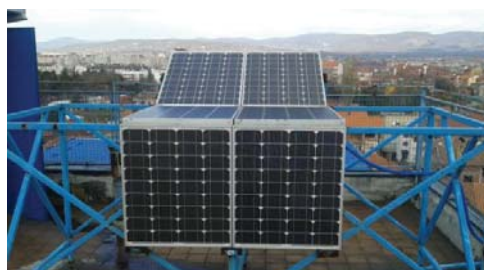
Figure 1. Two identical monocrystalline silicon solar modules ISF-60/12 on the roof of the Faculty of Science and Mathematics in Nis, used in the experiment
