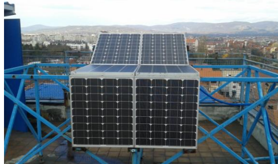
Fig. 1. Two identical monocrystalline silicon solar modules ISF-60/12 on the roof of the Faculty of Science and Mathematics in Nis, used in the experiment
