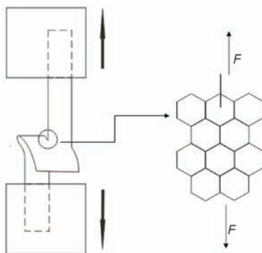
Figure 4. The single-rip tearing process
