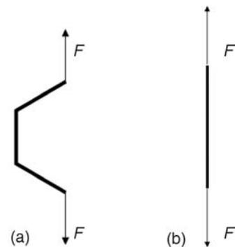
Figure 8. The deformation of the Steiner tree structure (a) before and (b) after damage
