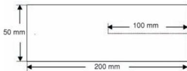
Figure 3. The sample for the single-rip tearing
