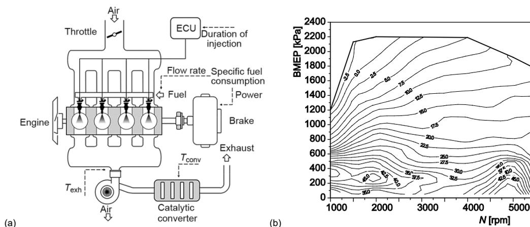
**Figure 1. Schematic representation of the experimental set-up and points of measurement for the chosen parameters (a) and map of spark timing setting (b)**
