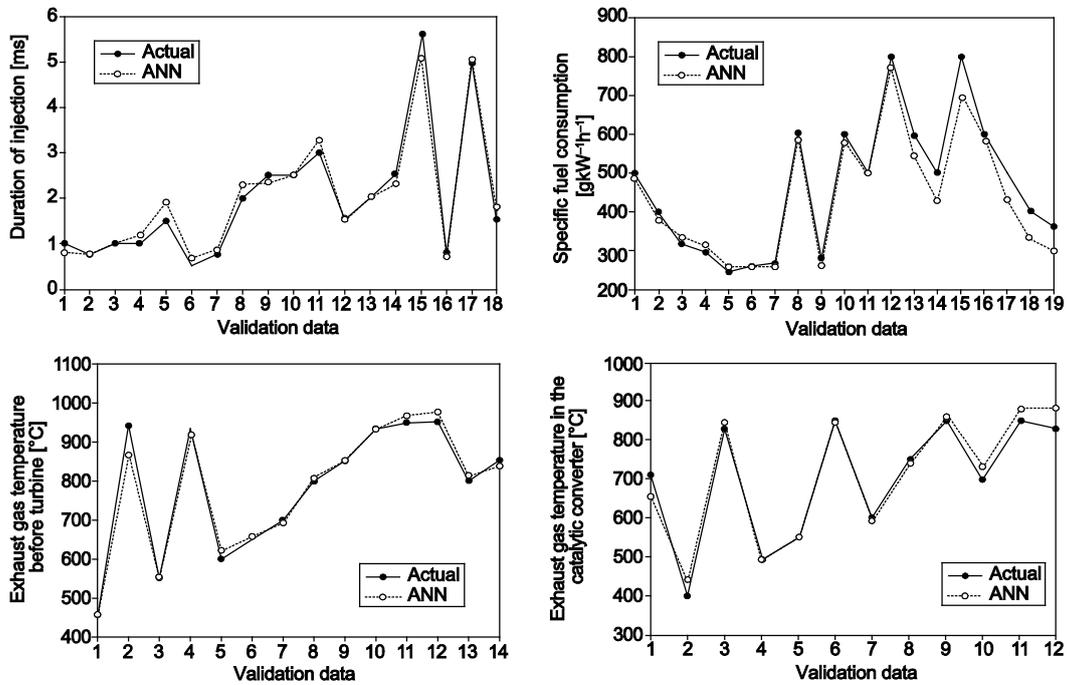
Figure 6. Validation results of DOI, SFC, exhaust gas temperature before turbine, and in the catalytic converter brick
