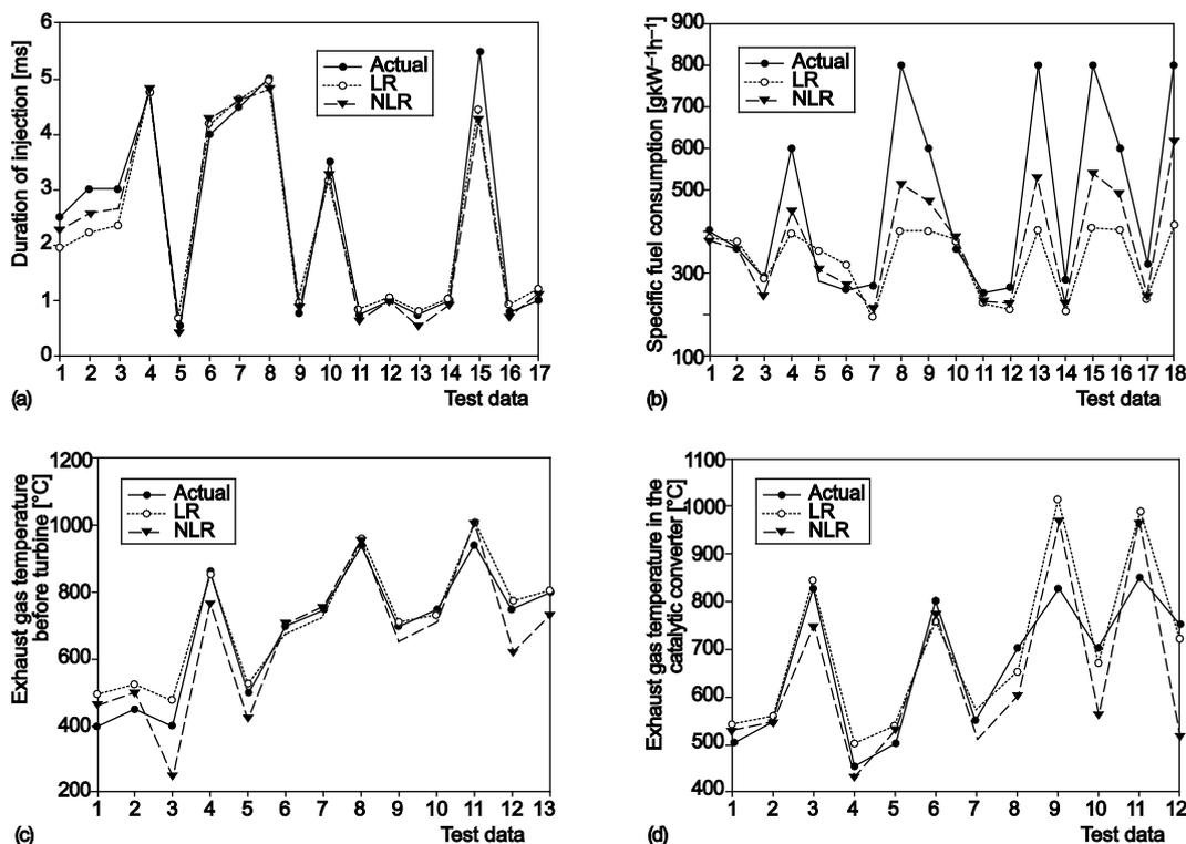
Figure 4. Comparison of actual and regression results of DOI, SFC, exhaust gas temperature before turbine, and in the catalytic converter brick
