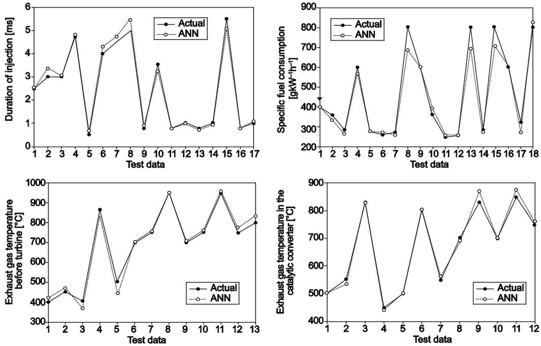
Figure 5. Testing results of actual and ANN results of DOI, SFC, exhaust gas temperature before turbine, and in the catalytic converter brick
