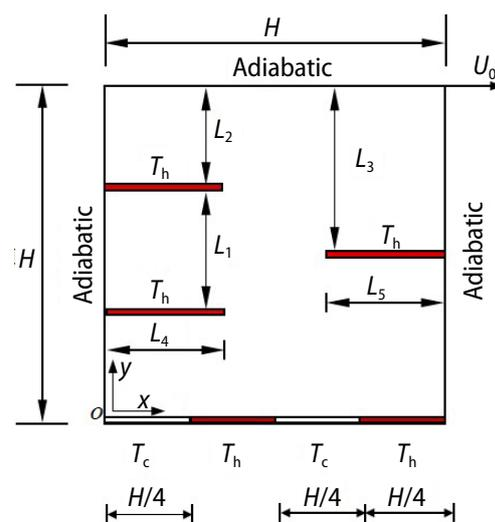
Figure 1. Schematic diagram of cavity with hot baffles
