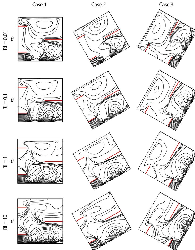
**Figure 2(b). Isotherms of COOH-functionalized DWCNT-water at different inclination angles and Richardson numbers at nanoparticles volume fraction of 0.004**
