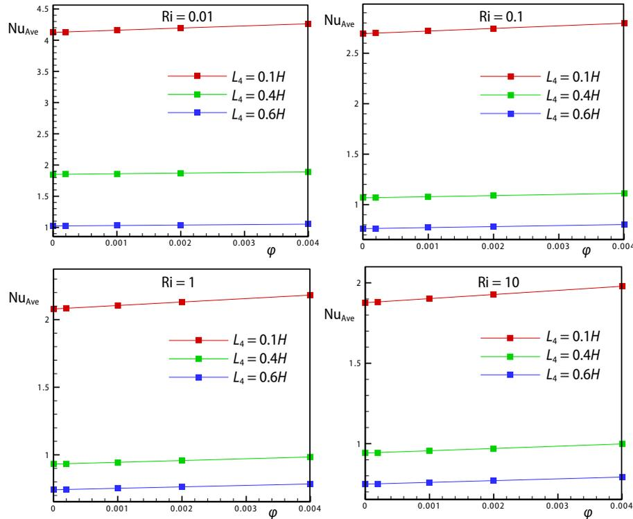
Figure 4. The variation of average Nusselt number vs. nanoparticles volume fraction at different Richardson numbers for different lengths ( $L_4$ ) of the left hot baffles
