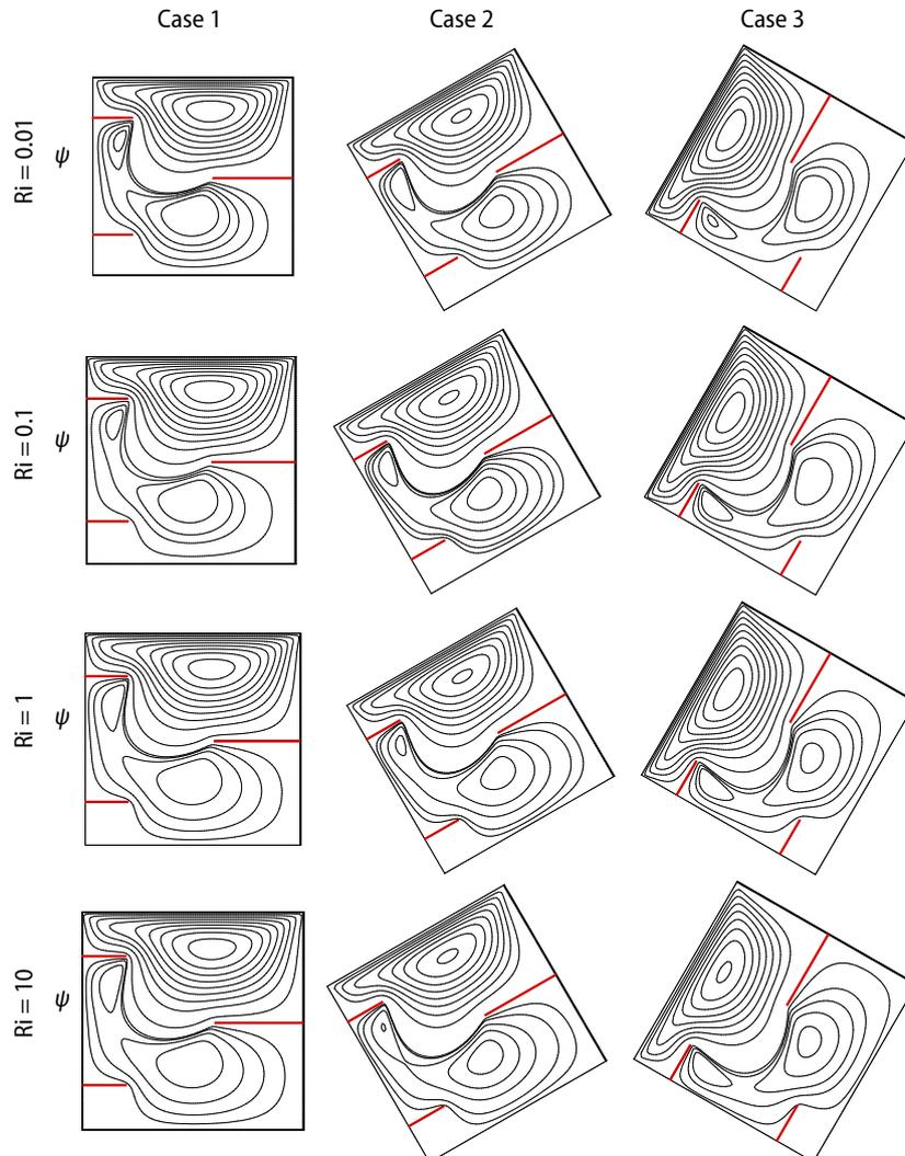
**Figure 2(a). Streamlines of COOH-functionalized DWCNT-water at different inclination angles and Richardson numbers at nanoparticles volume fraction of 0.004**
