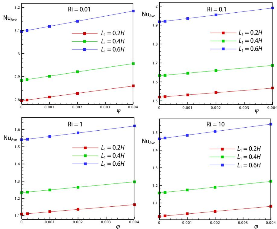
**Figure 3. The variation of average Nusselt number vs. nanoparticles volume fraction at different Richardson numbers at different ( $L_1$ ) between the left hot baffles**
