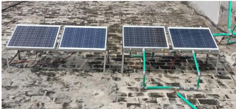
Figure 1 (a) Experimental setup: PV modules with cooling and without cooling
