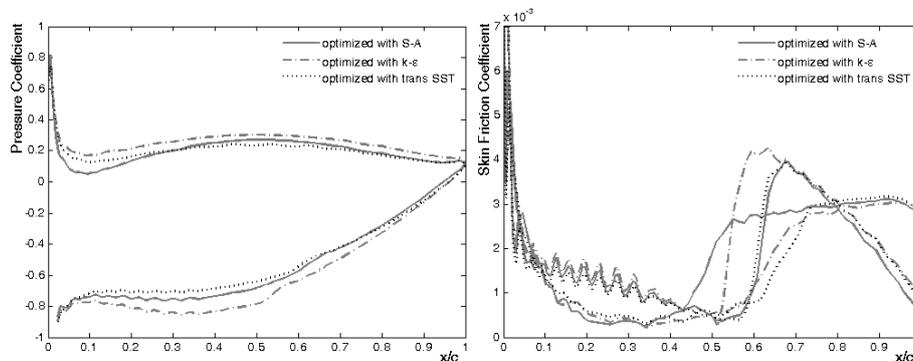
**Figure 9. Pressure and skin friction coefficients for all optimized airfoils obtained with the use of transitional SST**
