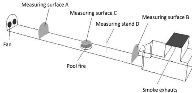
Figure 1. Basic geometry and measuring surfaces in the fire tunnel [7]
