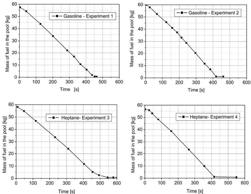
Figure 5. Changes of the fuel mass in the pool during the experiment [8]
