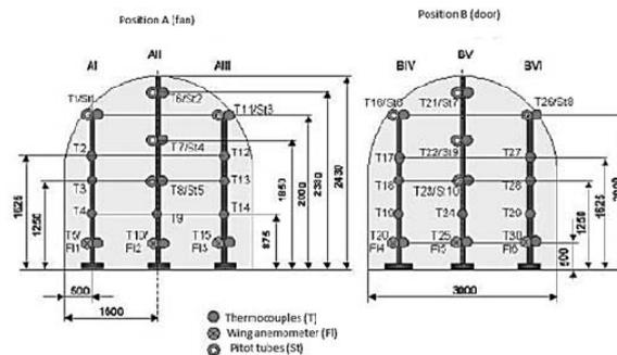
Figure 2. Illustration of measurement points on the measuring surfaces A and B [8]
