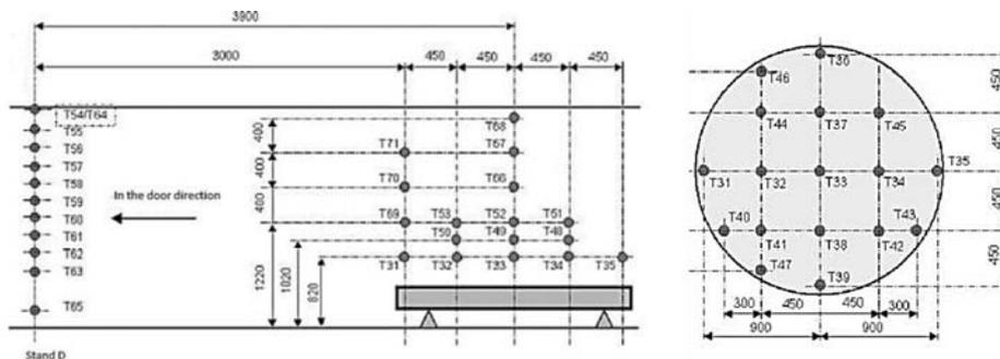
Figure 3. Schematic view of the thermocouples on the measuring surface C, directly above the pool and on the measuring surface D [8]
