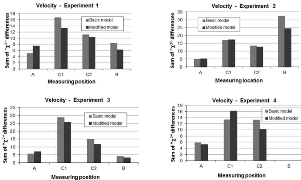
Figure 9. Comparison of deviation of experimental results from all 4 experiments for gas velocity values, with the results obtained by numerical simulation with basic and corrected package of CFD models, through the display of value of the sum of  $\chi^2$  differences
