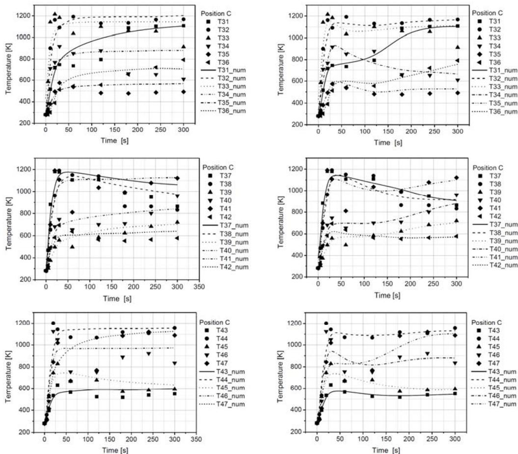
Figure 6. Comparison of experimental results and results of numerical simulations of air temperature changes along the tunnel axis at the measuring surface C, using the basic and corrected model for the first experiment
