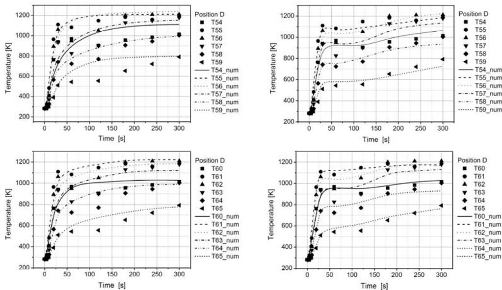
**Figure 7. Comparison of experimental results and results of numerical simulations of air temperature changes in the tunnel axis at the measuring position D, using the basic and corrected model for the first experiment**
