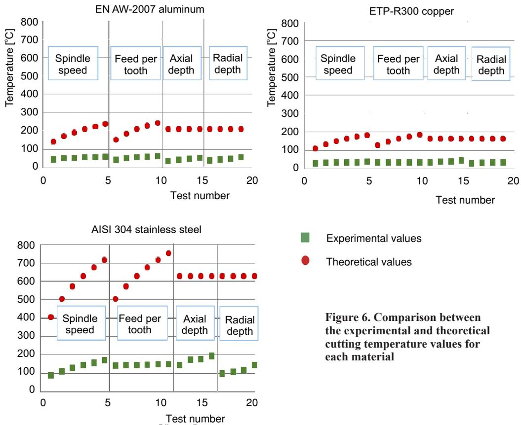
**Figure 6. Comparison between the experimental and theoretical cutting temperature values for each material**
