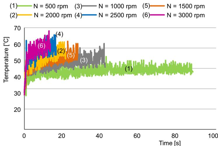
**Figure 3. Example of real temperature data collection of a milling process of an aluminum alloy workpiece by varying spindle speed; machining parameters:  $fz = 0.075 \text{ mm/tooth}$ ,  $a_p = 1$ ,  $a_e = 10 \text{ mm}$**
