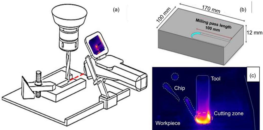
Figure 2. (a) position of the camera, tool, and workpiece, (b) schematic view of a sample cutting test, (c) example of the thermal image of a workpiece obtained with some details during milling
