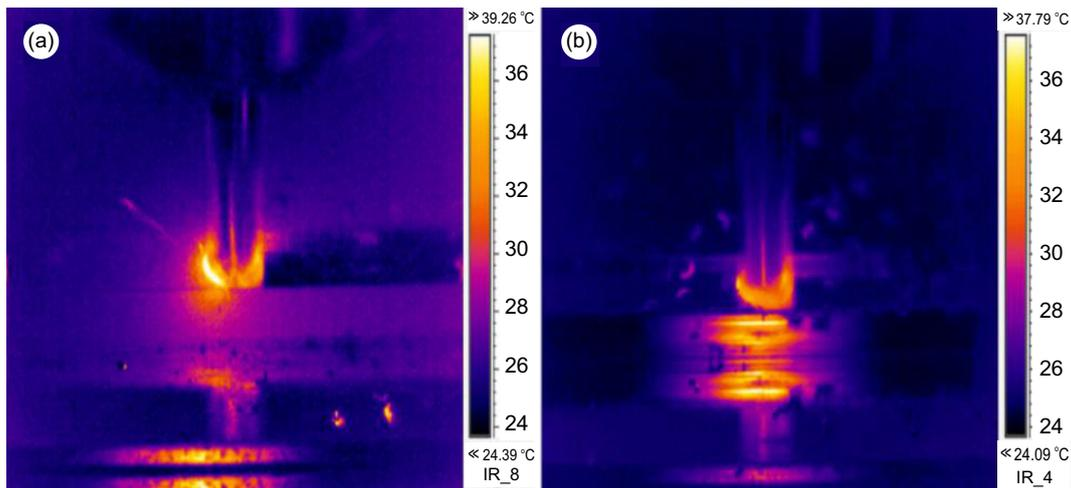
Figure 1. Thermal images in copper ETP-R300 milling; black painted area (a), bare zone (b)
