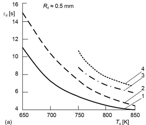
Figure 7. Ignition delay times of OCWF on the low-inertia thermocouple junction (type S, temperature measurement range is 273-1873 K, systematic error is  $\pm 1$  K, inertia is not more than 1 second, diameter of junction is about 0.1 second) depending on  $T_g$  (a) and  $R_d$  (b)
