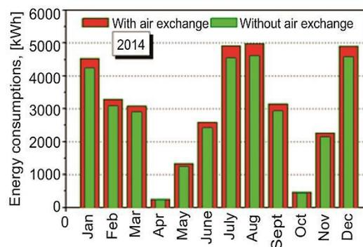
**Figure 7. Monthly energy needs for space heating and cooling**
