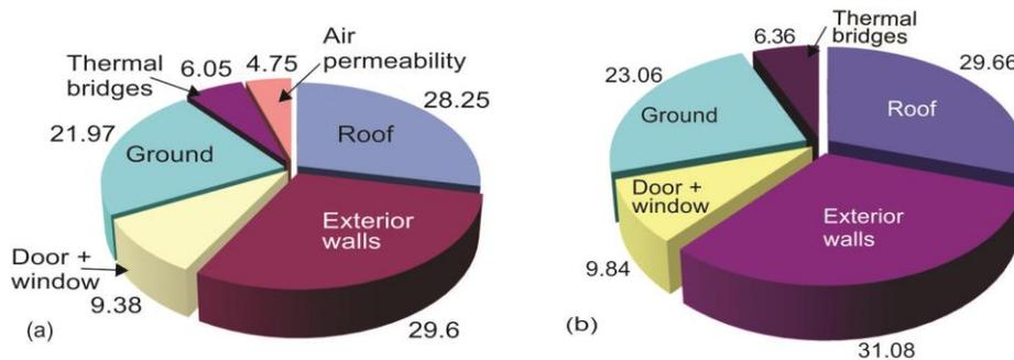
**Figure 6. Energy assessment of this real single-family house (by percentage of total losses); (a) permeable house to the air, (b) perfectly tight house**
