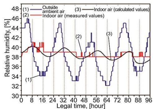
Figure 3. Relative humidity of the ambient and indoor air
