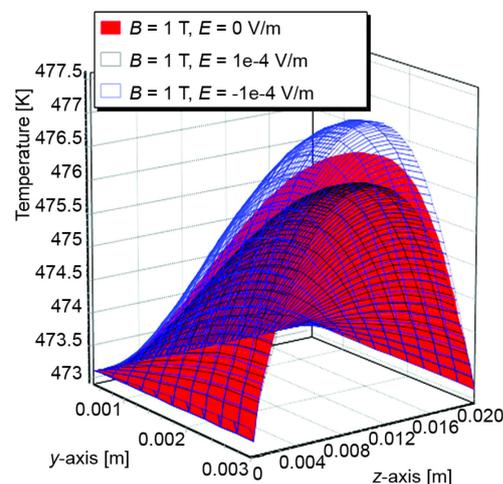
**Figure 5. Local temperature profile at  $z = 0.12$  m for  $B = 1$  T**
