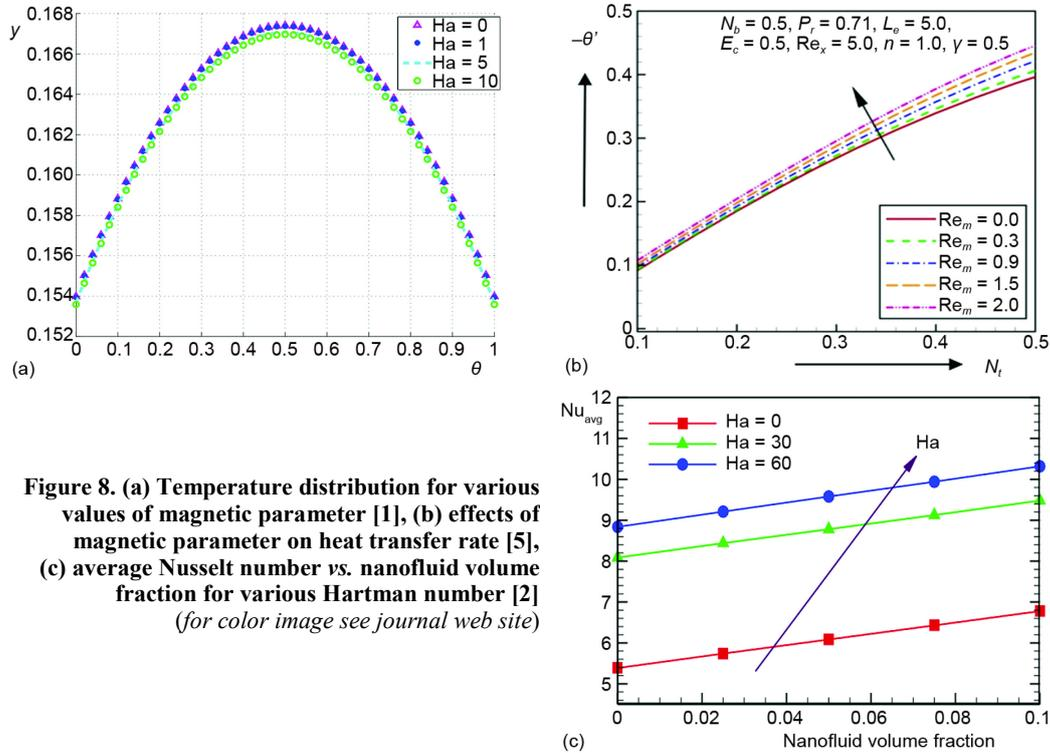
Figure 8. (a) Temperature distribution for various values of magnetic parameter [1], (b) effects of magnetic parameter on heat transfer rate [5], (c) average Nusselt number vs. nanofluid volume fraction for various Hartman number [2] (for color image see journal web site)
