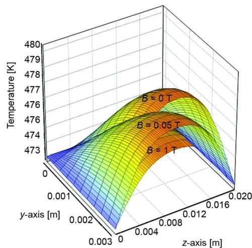
**Figure 3. Temperature profile at  $z = 0.12$  m** (for color image see journal web site)
