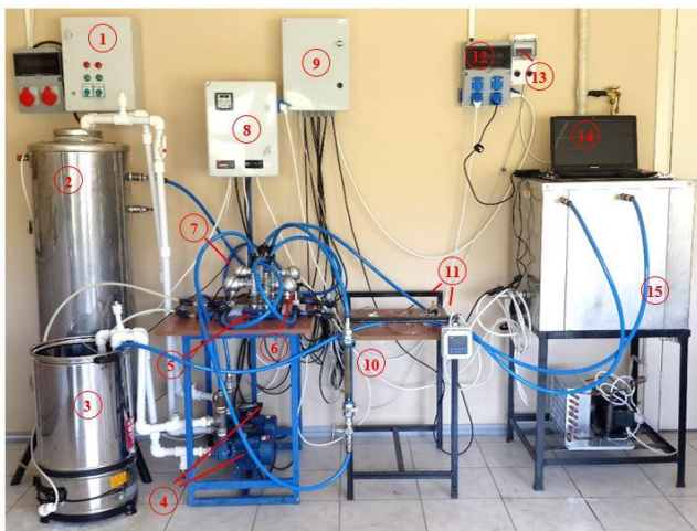
1. Power panel, 2. Hot water tank, 3. Nanofluid tank, 4. Pumps, 5. Test section, 6. Pressure difference, 7. Thermocouples, 8. Hot water tank temperature indicator and frequency control panel of pumps, 9. Data logger, 10. Hot water flow meter, 11. Cold nanofluid flow meter and indicator, 12. Power panel, 13. Nanofluid temperature control and indicator, 14. Computer, 15. Chiller.
