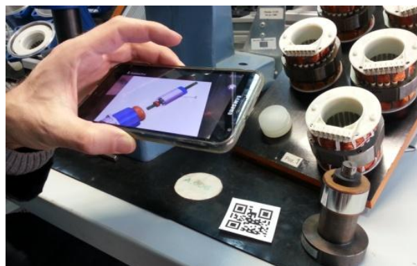
Figure 3. The AR interactive instructions for the disassembly sequence
